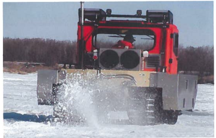
One of seven ice-cutting machines.
